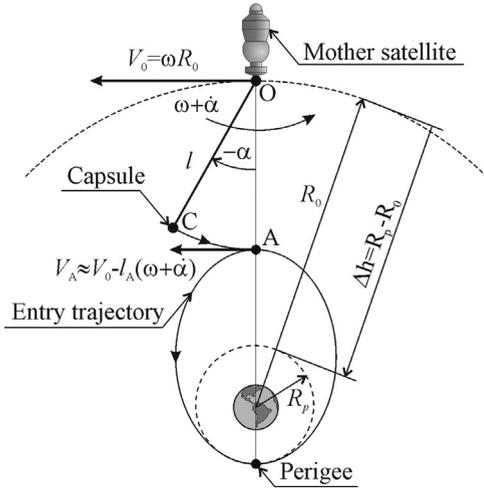
Fig. 1. Swinging release of a capsule from a tether.
