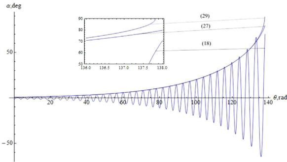
**Fig. 3.** The dependences of the deflection angle  $\alpha$  from true anomaly that are found using.
