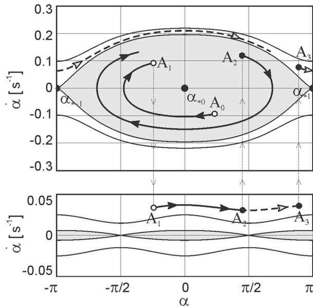
**Fig. 10** Transition phase trajectories through the separatrix at the weakening of the tether (point  $A_1$ ) and at re-tension (points  $A_2$  and  $A_3$ ); areas of oscillations bounded by separatrices are shown in gray
