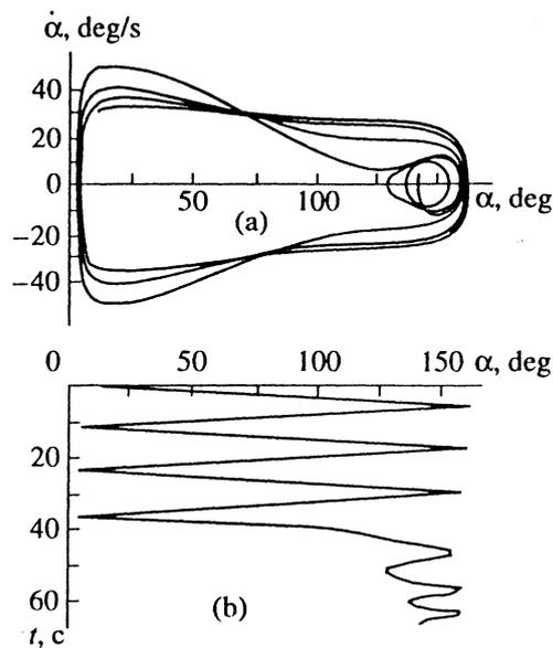
Fig. 5. Character of spatial motion variation during the reentry: (a) phase trajectories; (b) variation of the angle of attack.
