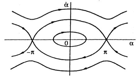
Fig. 1. Phase portrait of the planar motion:  $|a| \geq 2|b|$ .
