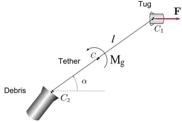
Fig. 1. Space debris and space tug connected by the tether
